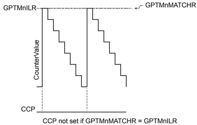
Figure 11-8 on page 707 shows how the CCP output operates when the `PLO` and `MRSU` bits are set and the `GPTMTnILR` is greater than the `GPTMTnMATCHR` value.
