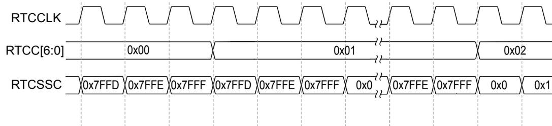
In the case of a trim value below `0x7FFF`, the `RTCSSC` value is advanced from `0x7FFF` to the trim value while the `RTCC` value is incremented from `0x0` to `0x1`. If the match value is within that range, the match interrupt is not triggered. For example, as shown in Figure 7-6 on page 485, if the match interrupt was configured with `RTCM0=0x1` and `RTCSSM=0x2`, an interrupt would never be triggered.
