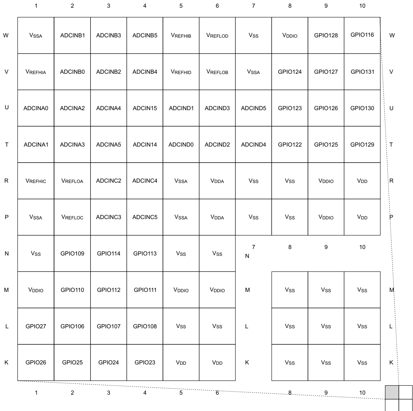
Figure 5-1. 337-Ball ZWT New Fine Pitch Ball Grid Array (Bottom View) – [Quadrant A]
