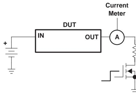
Figure 2. Current Limit Test Circuit
