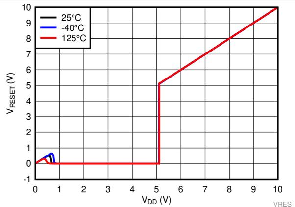
Figure 16. Output Voltage vs Input Voltage for TPS3840DL49
