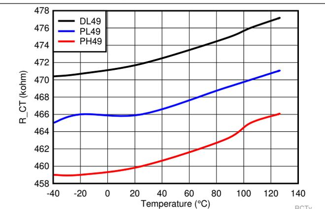
Figure 36. CT Pin Internal Resistance over Temperature
