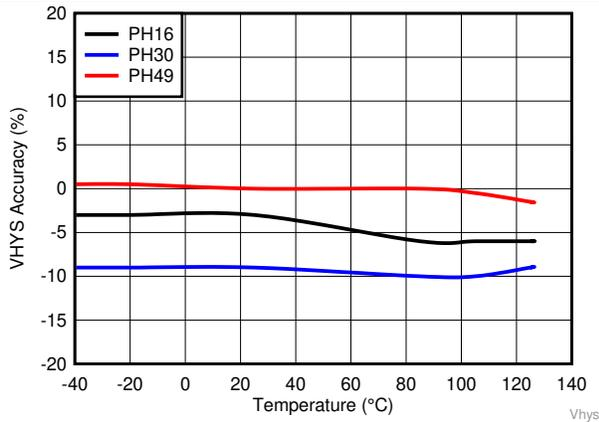
Figure 15. Input Threshold  $V_{IT}$ . Hysteresis Accuracy for TPS3840PHXX
