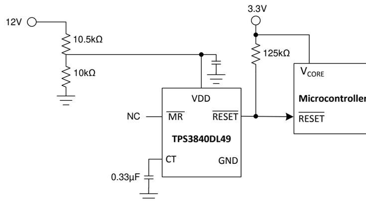
Figure 52. Fast Start Undervoltage Supervisor with Level-shifted Input
