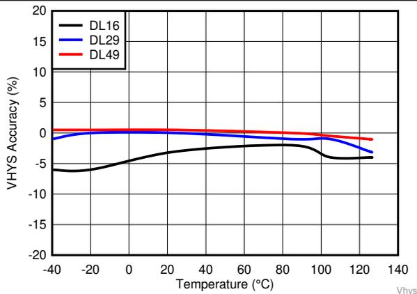
Figure 13. Input Threshold  $V_{IT}$ . Hysteresis Accuracy for TPS3840DLXX
