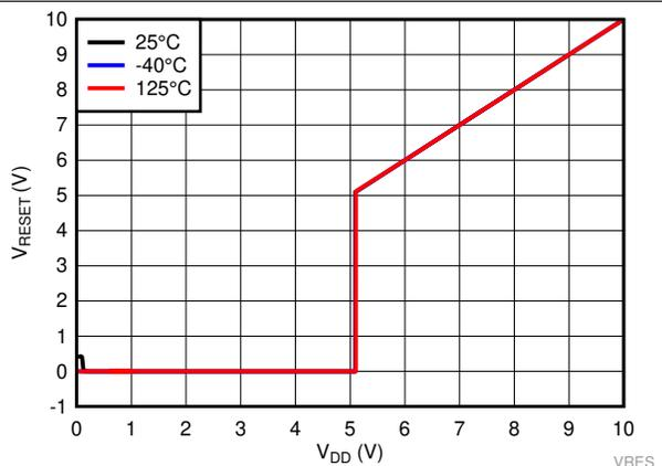
Figure 17. Output Voltage vs Input Voltage for TPS3840PL49
