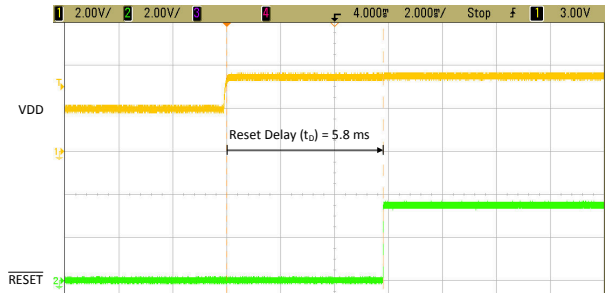
Figure 8-8. TPS3840EVM \overline{\text{RESET}} Time Delay ( t_D ) with 0.01- \mu\text{F} Capacitor
