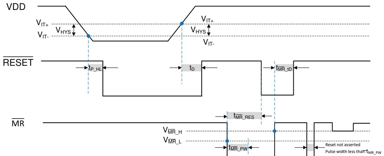
Figure 47. Timing Diagram  $\overline{\text{MR}}$  and  $\overline{\text{RESET}}$  (TPS3840DL)
