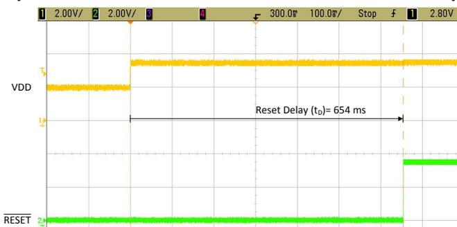
Figure 56. TPS3840EVM  $\overline{\text{RESET}}$  Time Delay ( $t_D$ ) with 1- $\mu\text{F}$  Capacitor
