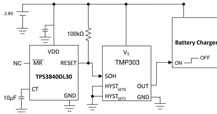
Figure 51. Overvoltage and Window Temperature Monitoring Solution
