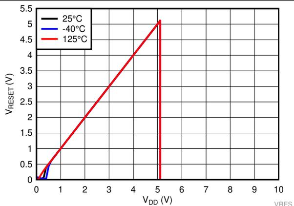
Figure 18. Output Voltage vs Input Voltage for TPS3840PH49
