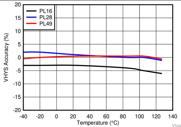
Figure 14. Input Threshold  $V_{IT}$ . Hysteresis Accuracy for TPS3840PLXX
