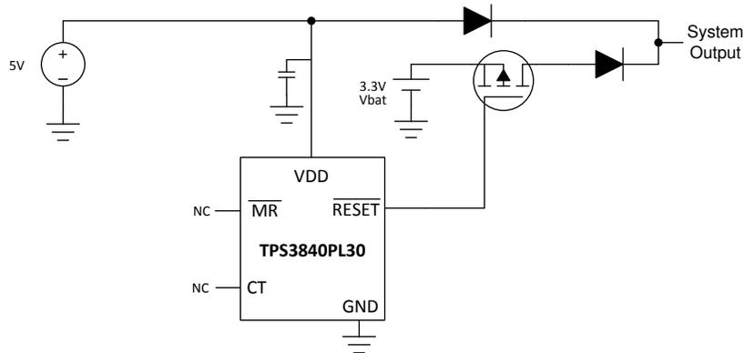
Figure 53. Voltage Monitor with Back-up Battery Switchover Solution
