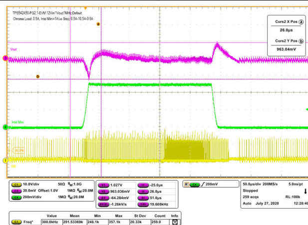
Figure 6-26. Load Transient 2 A to 12 A to 2 A at 20 A/μs
