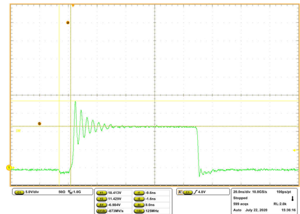
V_{IN} = 12\text{ V} V_{OUT} = 1\text{ V} f_{SW} = 1.0\text{ MHz} BOM Figure 6-22. Switch Node Ringing and Dead-Time at 10-A Output Current
