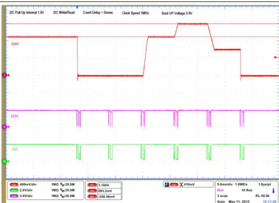
Figure 13. PMBus 1-MHz Bus Speed with 1.8-V Pullup
