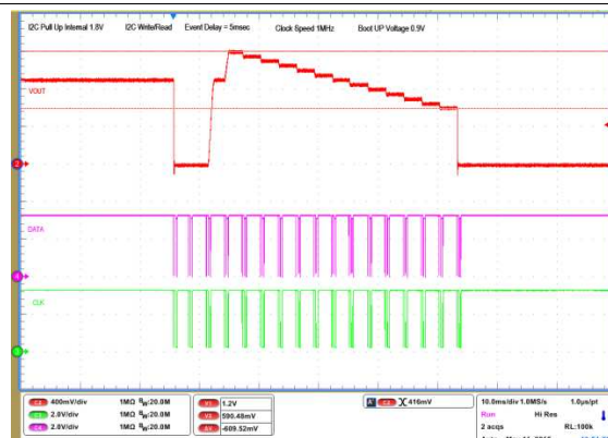
Figure 16. 6 Sequenced Events – I2C Write/Read with PEC
