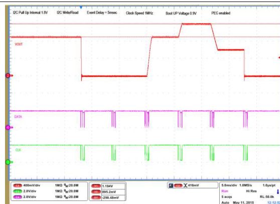
Figure 14. 6 Sequenced Events – I2C Write
