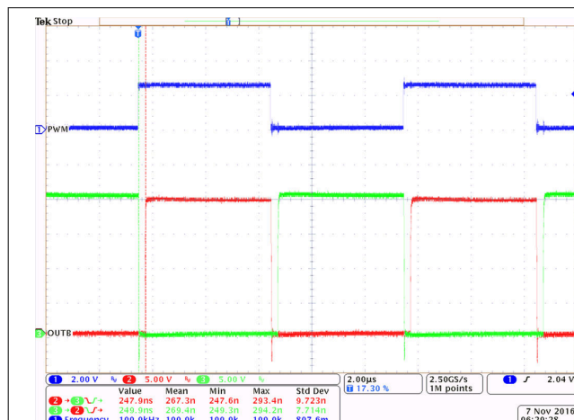
Figure 9-5. Bench Test Waveform for PWM and OUTA/B
