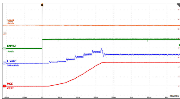
Figure 8-2. Start-Up with EN/FLT From Low to High: VINP = 5.0V, VCC = 5.0V, 18Ω Load
