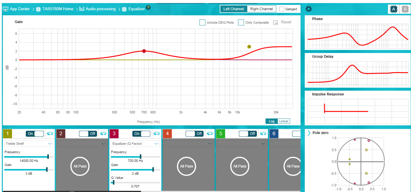
Figure 21. Equalizer Tuning Window
