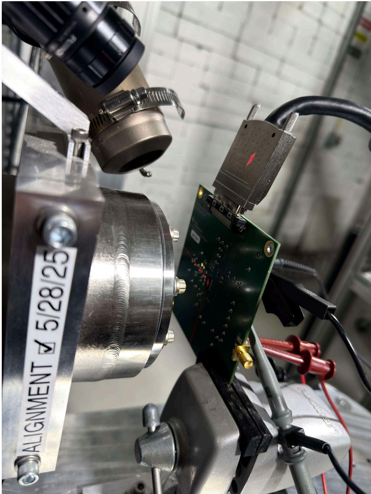
Figure 4-1. TPS7H503x-SP EVM in Front of the Heavy-Ion Beam Exit Port at the MSU KSEE Cyclotron
