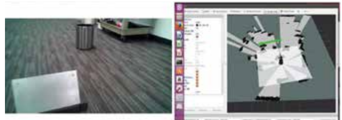
Figure 12. Using the IWR1443 EVM occupancy map for autonomous navigation of a Turtlebot 2 with the Robot OS move_base library.
