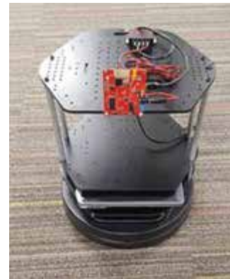
Figure 9. IWR1443 EVM mounted on a Turtlebot 2.
