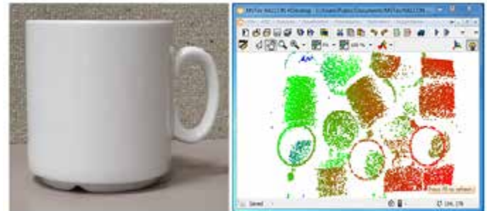
Figure 4. Captured mug (left) and acquired point cloud acquired with DLP® powered structured light of several mugs in a box displayed in Halcon HDevelop (right).
