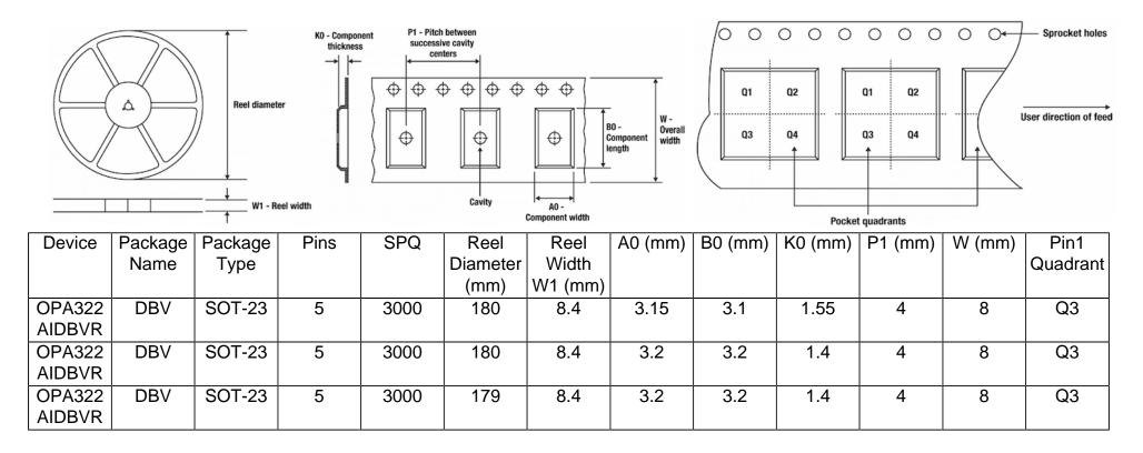
Images above are just a representation of the carrier. Actual carrier may vary. Please reference the dimensions provided in the table.
