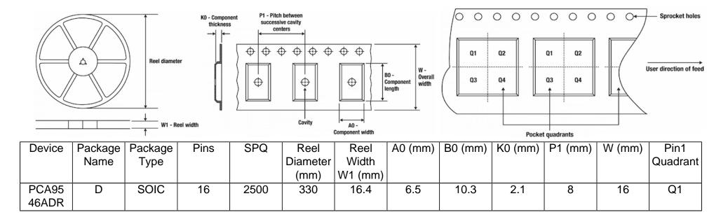
Images above are just a representation of the carrier. Actual carrier may vary. Please reference the dimensions provided in the table.
