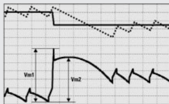
Figure 5. Typical load-current transient waveforms
