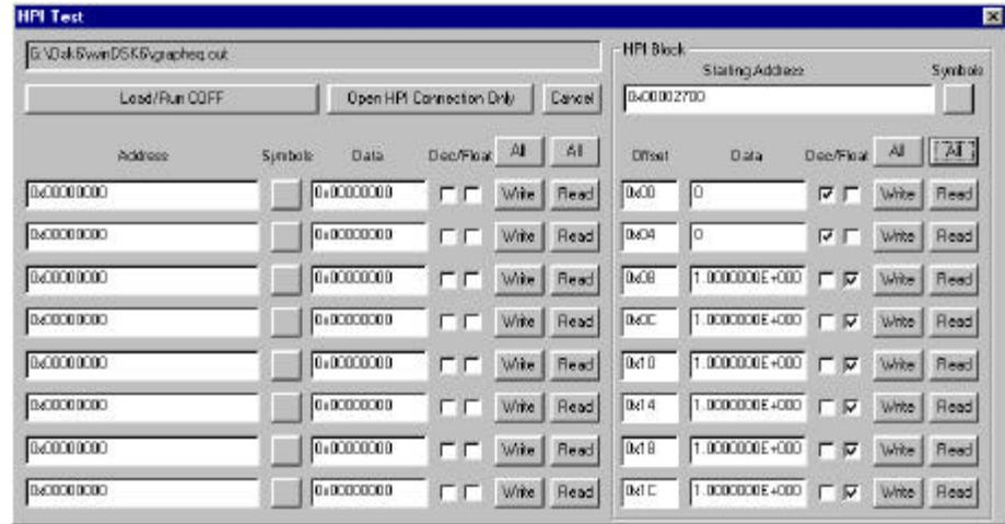
labels from a list. The data can be viewed, edited, and written in floating or integer forms. The HPI Test is particularly useful for modifying memory when reading and writing must be done independently, a function that is not available under Code Composer.
