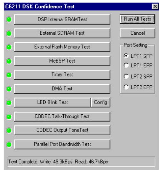
The DSK Confidence Test is an easy way to test the basic functionality of the DSK, providing a graphical interface to the confidence test supplied with DSK. Visual indicators show test progress and status. Each test may be run individually, or all can run in an automatic sequence. In addition, the DSK Confidence Test also tests and reports the speed of the parallel port connection between the host PC and the DSK in both directions.
