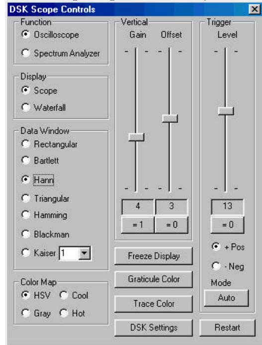
The oscilloscope / spectrum analyzer can operate as a standard oscilloscope or as a spectrum analyzer. The resizable display window can be viewed as a conventional oscilloscope, or a waterfall display can be selected with various colormaps. For spectral analysis, a number of different data windows can be selected. Standard oscilloscope triggering methods are also supported.
