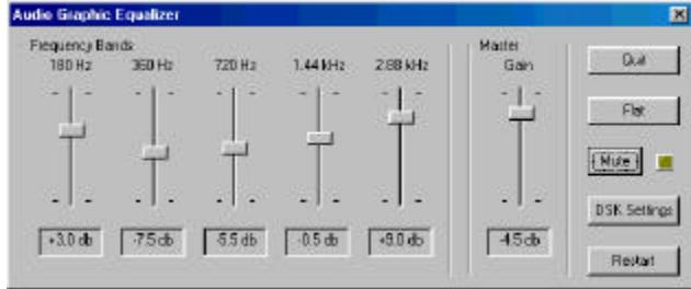
The five-band graphic equalizer uses five parallel 128<sup>th</sup> order FIR filters, with the gain of each filter independently controlled by a slider control. A master gain control, mute button, and flat button provide additional control.
