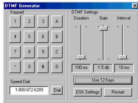
The DTMF generator can generate all 16 DTMF tone pairs. The duration of each tone, as well as the interval between tones, can be adjusted. A 12-key or 16-key keypad can be selected. A speed dial feature operates in the same way as a typical telephone.
