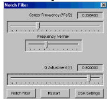
This application implements a single stage IIR filter acting as a notch or bandpass filter. The filter center frequency and Q can be adjusted.
