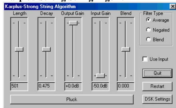
Implements the Karplus-Strong string algorithm [2] to synthesize a plucked string. The delay buffer length, decay coefficient, and the filter type are all user adjustable. Additionally, the ADC input can be processed through the algorithm by using it to excite the string buffer on a continuous basis.
