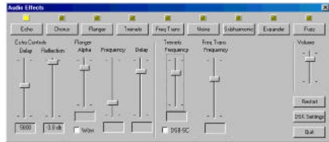
The audio effects application demonstrates a variety of signal manipulations possible using DSP, including echo, chorus, flanging, tremolo (amplitude modulation), noise, and frequency translation. Many of the effect parameters can be varied well beyond the customary values used with music to produce unusual effects.
