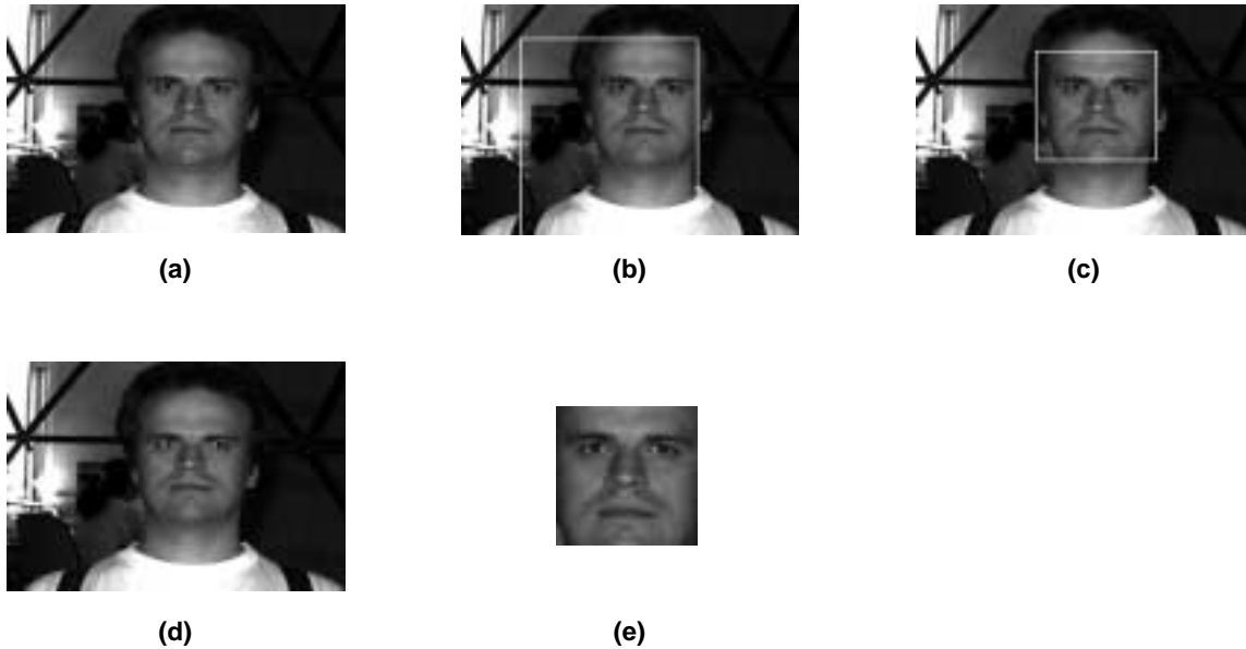
Figure 2. Face Detection, Eye Localization and Face Normalization Stages: (a) original image, (b) The box shows the reduced search space for the face after the rule-based technique is applied. At least half of the face is assumed to be inside these boundaries., (c) result of the face detection stage, (d) result of the eye localization stage, (e) normalized face image
