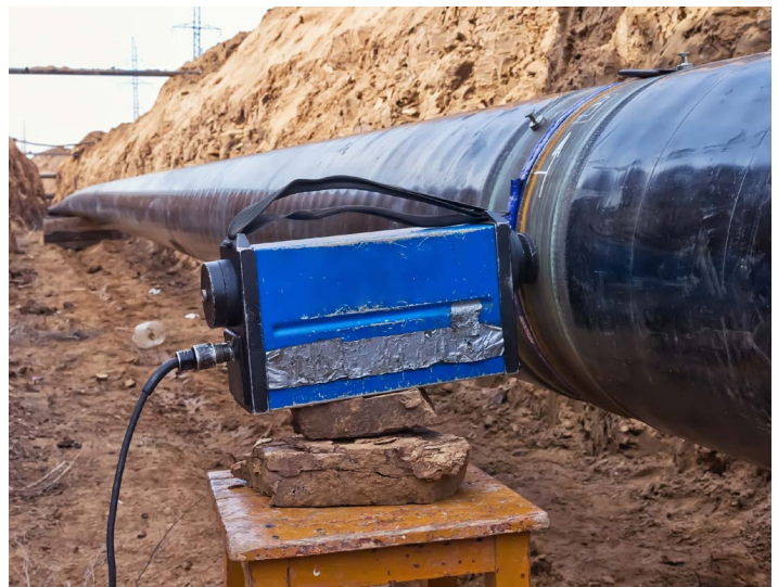
Figure 1-24. X-ray image of the contents of a bag in an airport security line (top); a portable X-ray machine to scan for pipe defects (bottom).
