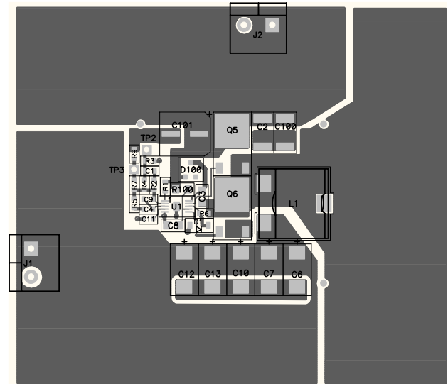
Fig. 34. Massive copper pours help spread heat.
