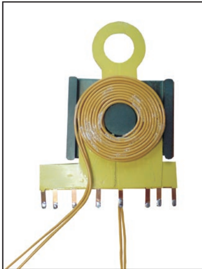
a. One half of transformer showing two primary coils in parallel, with center termination brought out along a groove (hidden) in the core face.
