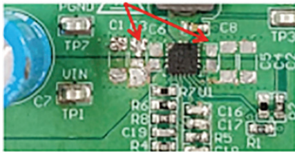
Figure 28 – Converter layout with no nearby input decoupling capacitor populated.
