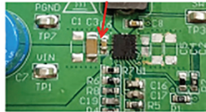
Figure 30 – Converter layout with two input capacitors populated right next to the IC.
