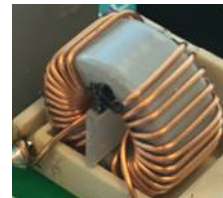
Figure 35 – Modified 1-layer split-wound CM filter choke.
