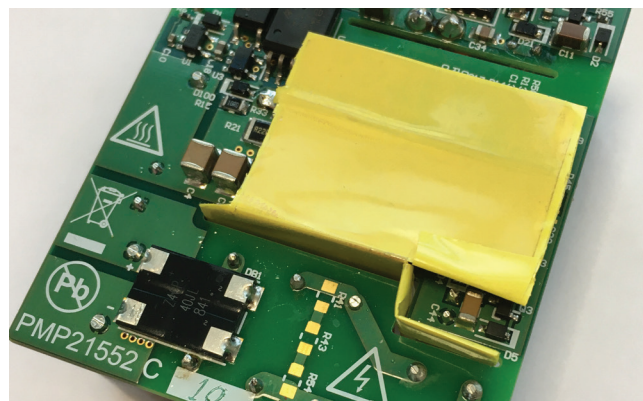
Figure 26 – Circuit shielding example.
