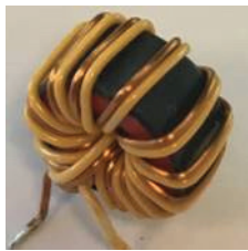
Figure 33 – Example bifilar-wound, 1-layer CM filter choke.
