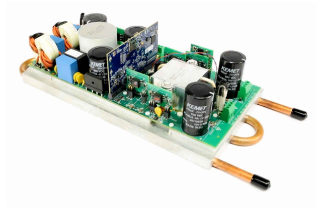
Figure 44. 6.6-kW OBC with liquid-cooled cold plate.
