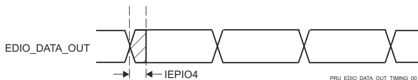
Figure 6-114. PRUSS IEP Digital IOs Timing Requirements
