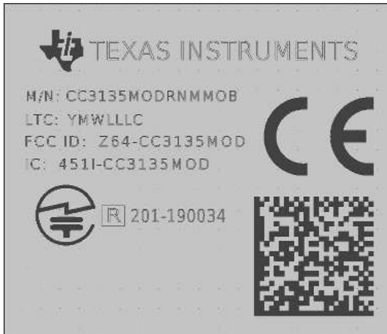
Figure 8-1. SimpleLink™ CC3135 Module Markings
