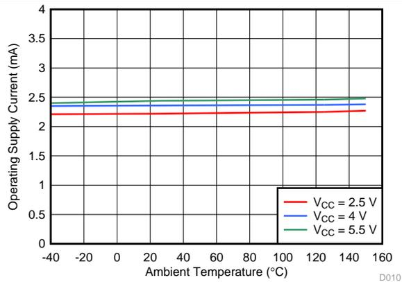
Figure 10.  $I_{CC}$  vs Temperature (DRV5015A2, DRV5015A3)
