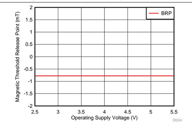
Figure 4.  $B_{RP}$  Threshold vs Supply Voltage (DRV5015A1)
