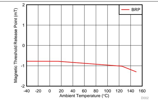
Figure 2.  $B_{RP}$  Threshold vs Temperature (DRV5015A1)
