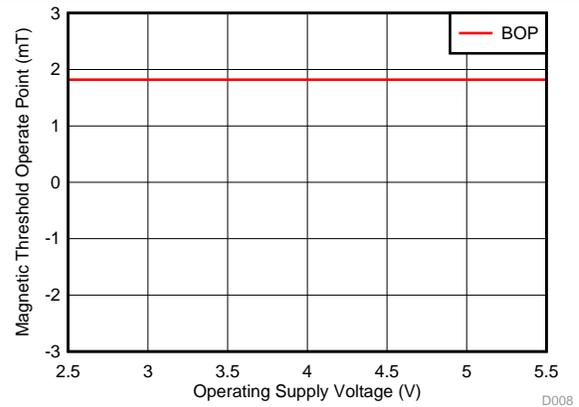
Figure 8.  $B_{OP}$  Threshold vs Supply Voltage (DRV5015A2, DRV5015A3)
