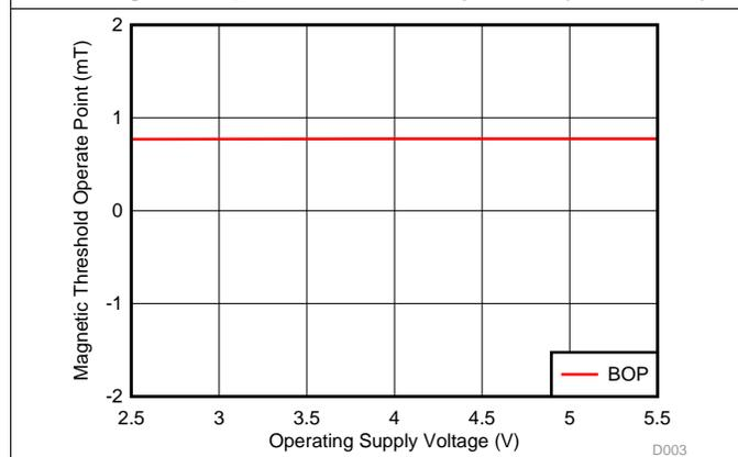
Figure 3.  $B_{OP}$  Threshold vs Supply Voltage (DRV5015A1)
