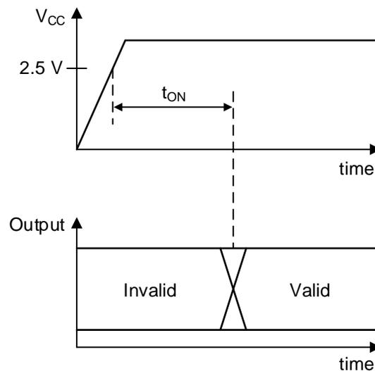
Figure 15.  $t_{ON}$  Definition
