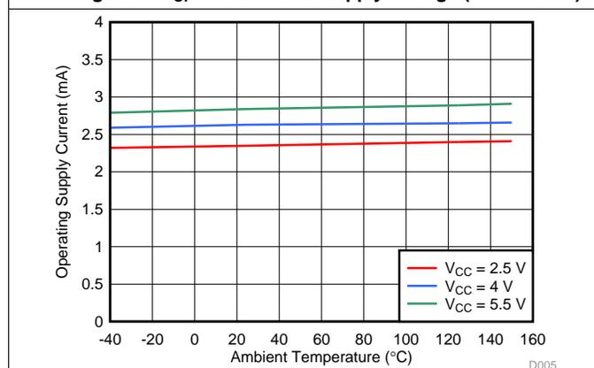
Figure 5.  $I_{CC}$  vs Temperature (DRV5015A1)
