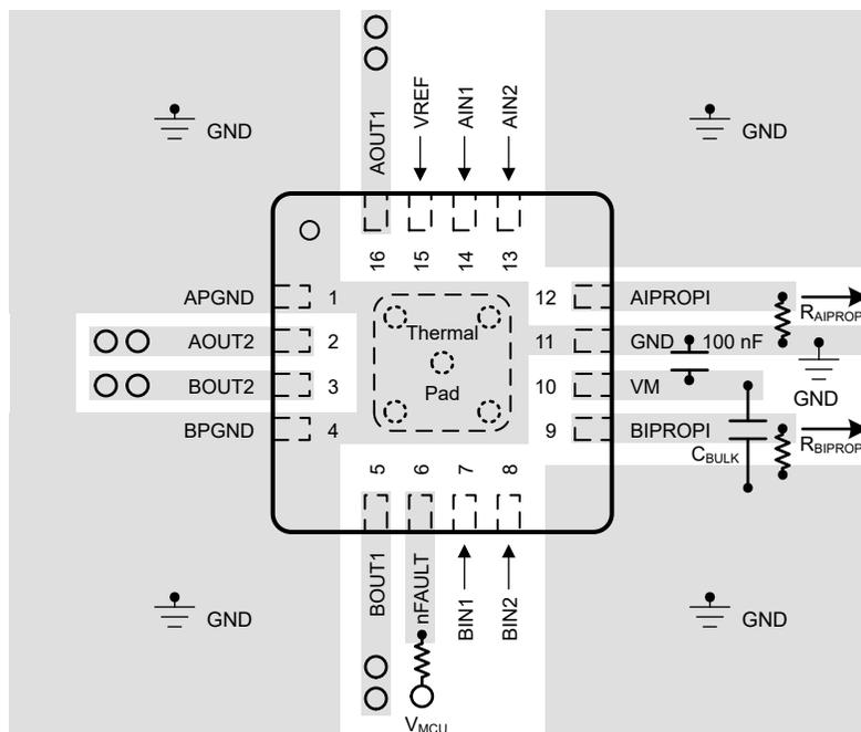
Figure 9-23. Recommended Layout Example for RTE (WQFN) Package
