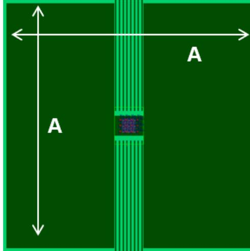
Figure 9-11. HTSSOP PCB model top layer
