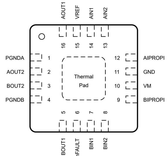
**Figure 5-2. RTE Package 16-Pin WQFN Top View**
