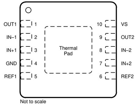
A. Thermal Pad can be left floating or connected to GND.
