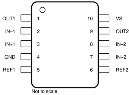
**Figure 5-3. INA2181: DGS Package 10-Pin VSSOP Top View**
