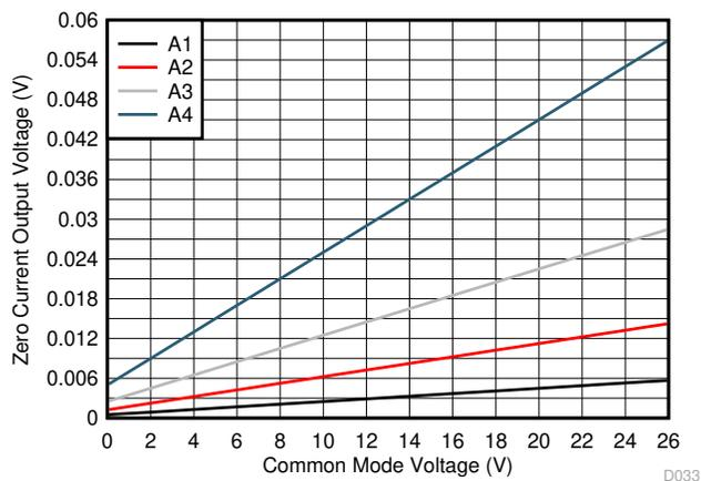
Figure 7-5. Zero-Current Output Voltage vs Common-Mode Voltage
