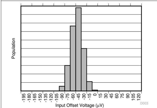
Figure 6-3. Input Offset Voltage Production Distribution A3
