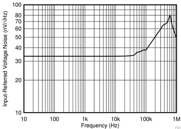
**Figure 6-29. Input-Referred Voltage Noise vs Frequency (A3 Devices)**
