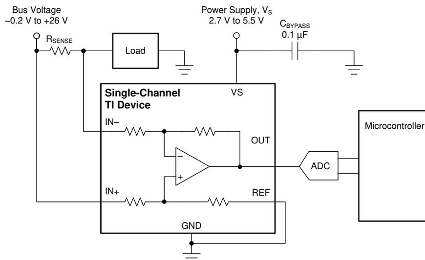
NOTE: To help eliminate ground offset errors between the device and the analog-to-digital converter (ADC), connect the REF pin to the ADC reference input and then to ground. For best performance, use an RC filter between the output of the INAx181 and the ADC. See [Closed-Loop Analysis of Load-Induced Amplifier Stability Issues Using ZOUT](#) application note for more details.
