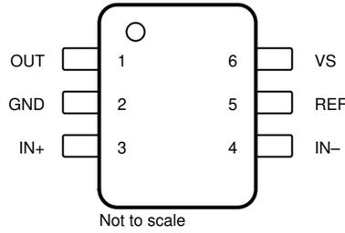
Figure 5-1. INA181: DBV Package 6-Pin SOT-23 Top View
