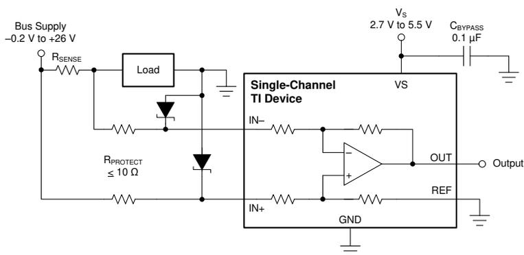
**Figure 8-9. Transient Protection Using Dual Zener Diodes**
