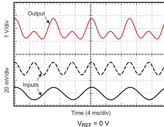
**Figure 8-4. Current Summing Application Output Response (A2 Devices)**
