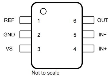
Figure 5-2. INA181: DCK Package 6-Pin SC70 Top View
