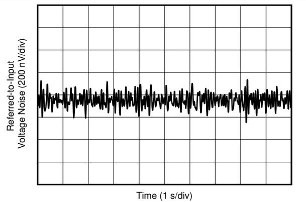
**Figure 6-30. 0.1-Hz to 10-Hz Voltage Noise (Referred-to-Input)**
