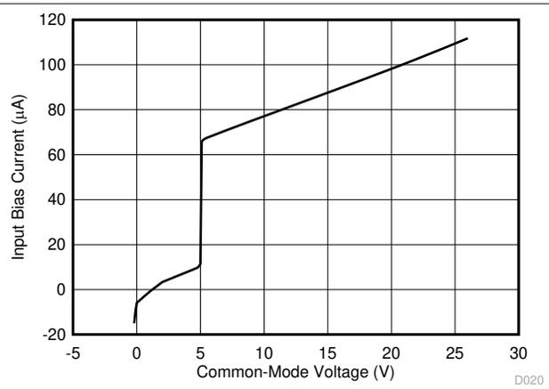
**Figure 6-20. Input Bias Current vs Common-Mode Voltage**
