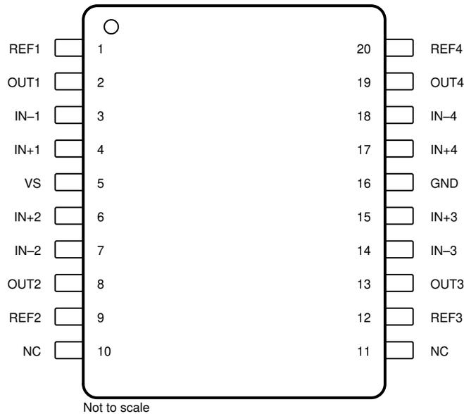
**Figure 5-5. INA4181: PW Package 20-Pin TSSOP Top View**
