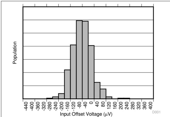
Figure 6-1. Input Offset Voltage Production Distribution A1
