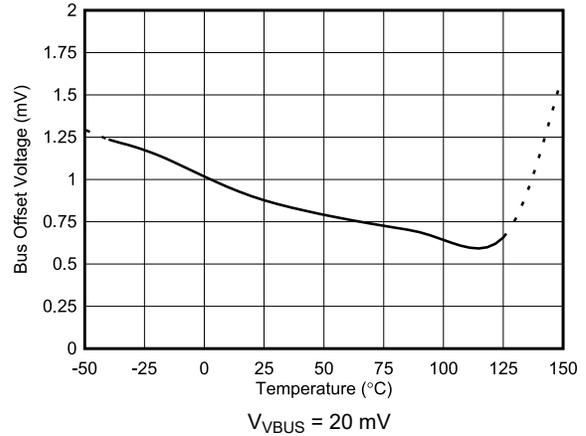
**Figure 6-11. Bus Input Offset Voltage vs. Temperature**
