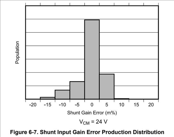
Figure 6-7. Shunt Input Gain Error Production Distribution
