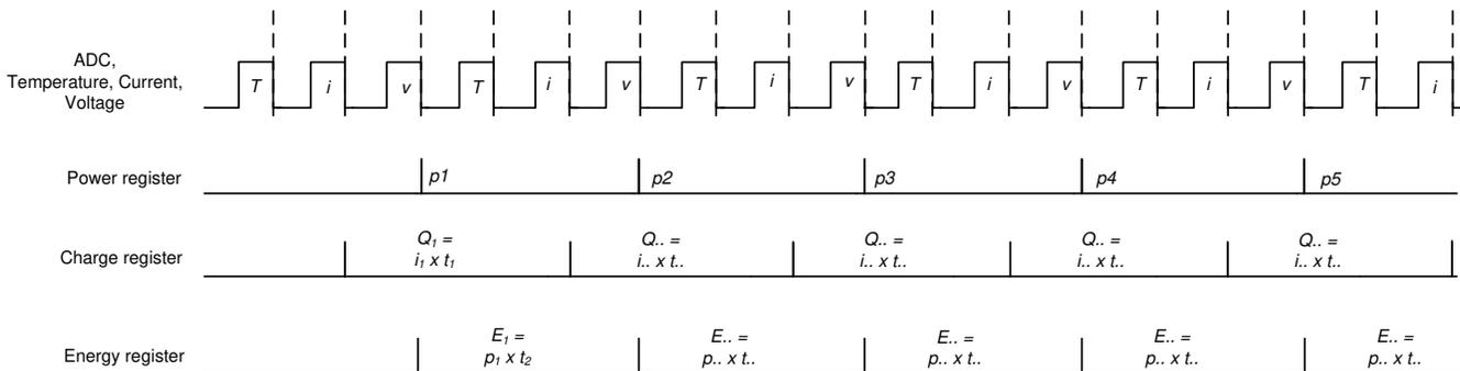
**Figure 7-2. Power, Energy and Charge Calculation Scheme**
