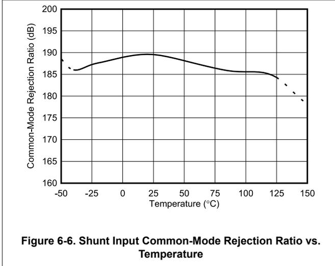
Figure 6-6. Shunt Input Common-Mode Rejection Ratio vs. Temperature
