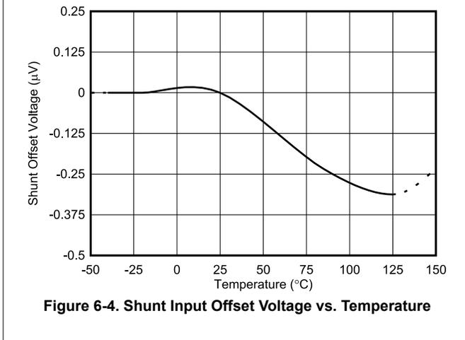
Figure 6-4. Shunt Input Offset Voltage vs. Temperature
