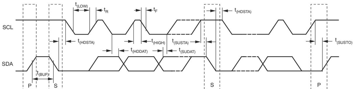
Figure 6-1. I<sup>2</sup>C Timing Diagram
