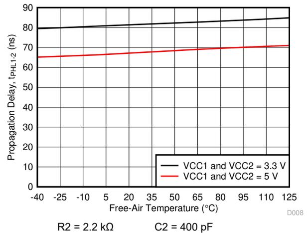
Figure 6-11.  $t_{PHL1-2}$  Propagation Delay vs Free-Air Temperature
