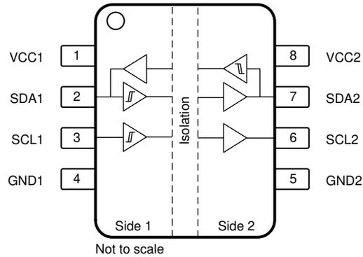
**Figure 5-2. ISO1541 D Package 8-Pin SOIC Top View**
