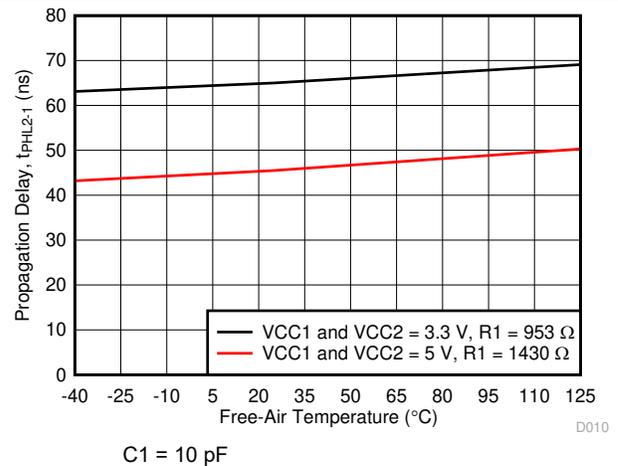
Figure 6-13.  $t_{PHL2-1}$  Propagation Delay vs Free-Air Temperature
