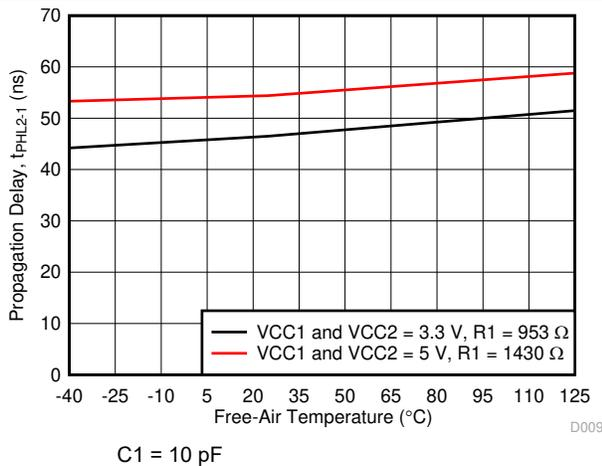
Figure 6-12.  $t_{PLH2-1}$  Propagation Delay vs Free-Air Temperature
