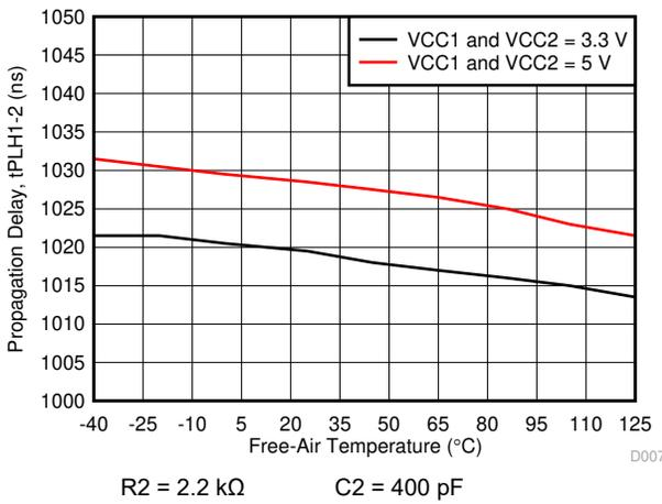
Figure 6-10.  $t_{PLH1-2}$  Propagation Delay vs Free-Air Temperature
