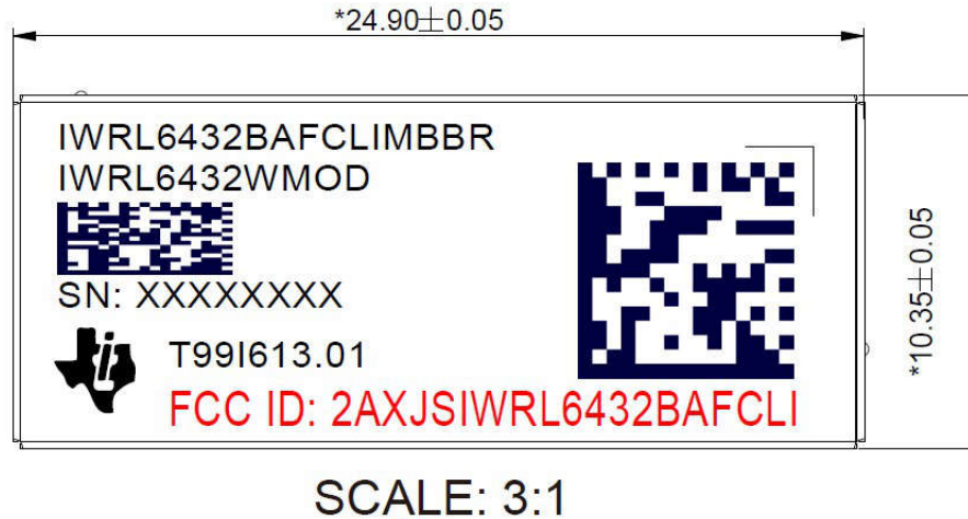
Figure 9-3. Example of Device Part Markings
