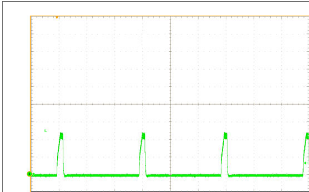
Figure 8-18. Inductor Current Bursts During Hiccup
