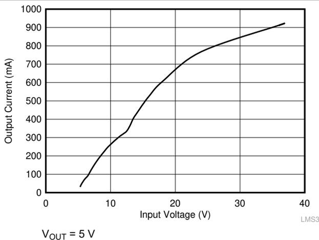
Figure 9-9. Load Current for PFM-to-PWM Transition
