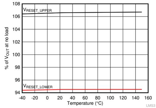
**Figure 7-8. RESET Threshold as Percentage of Output Voltage**
