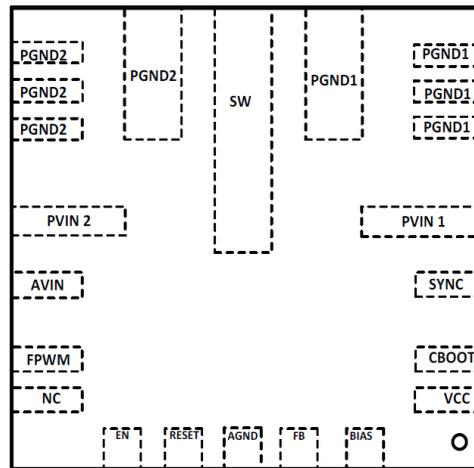
Figure 6-1. RNL Package 22-Pin VQFN Top View
