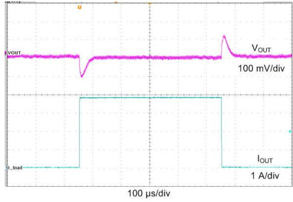
FPWM                       $V_{OUT} = 6 V (ADJ)$                        $L = 10 \mu H,$
