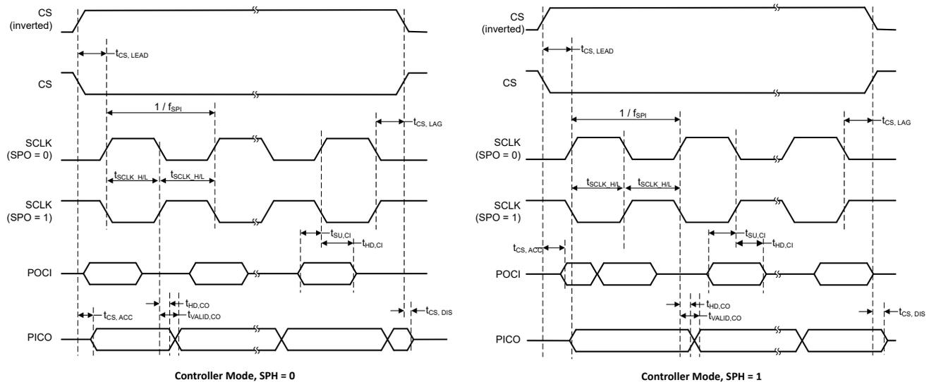
Figure 7-4. SPI Timing Diagram - Controller Mode
