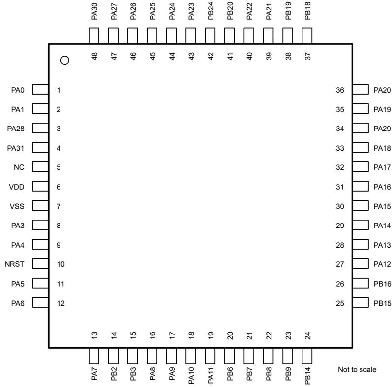
**Figure 6-3. 48-pin PT (B) (LQFP) Package**
