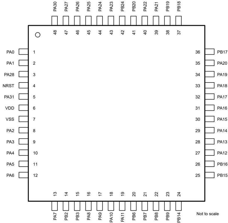
**Figure 6-2. 48-pin PT (A) 48-pin PT (LQFP) Package**
