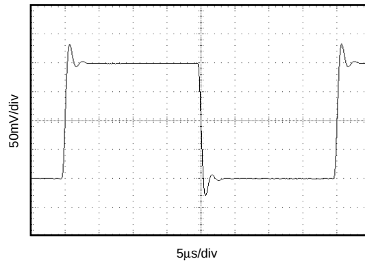
OPA704 SMALL SIGNAL STEP RESPONSE ( G = +5\text{V/V} , C_F = 3\text{pF} , R_F = 100\text{k}\Omega , C_L = 100\text{pF} , R_L = 20\text{k}\Omega )
