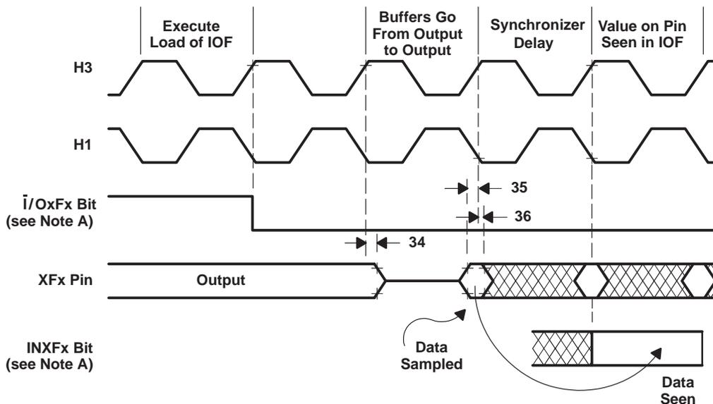
NOTE A:  $\bar{I}/OxFx$  represents either bit 1 or bit 5 of the IOF register, and  $INxFx$  represents either bit 3 or bit 7 of the IOF register.
