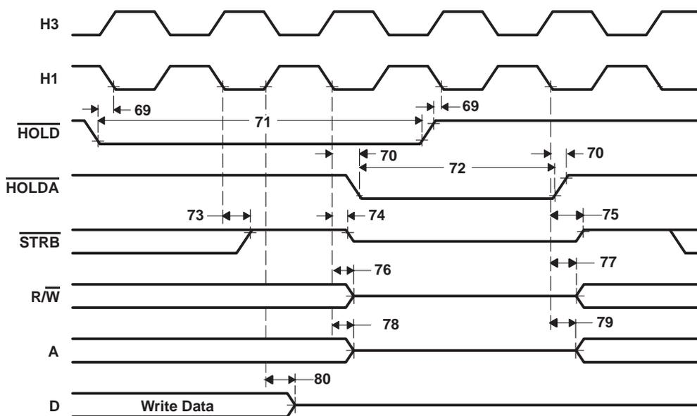
NOTE A:  $\overline{\text{HOLDA}}$  goes low in response to  $\overline{\text{HOLD}}$  going low and continues to remain low until one H1 cycle after  $\overline{\text{HOLD}}$  goes back high.
