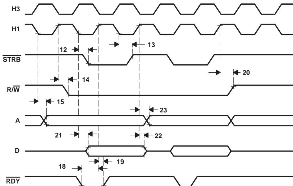
Figure 15. Timing for Memory ( $\overline{\text{STRB}} = 0$ ) Write
