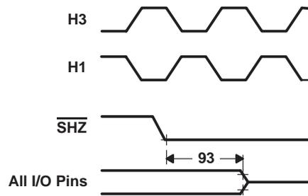
NOTE A: Enabling  $\overline{\text{SHZ}}$  destroys SMJ320C3x register and memory contents. Assert  $\overline{\text{SHZ}} = 1$  and reset the SMJ320C3x to restore it to a known condition.
