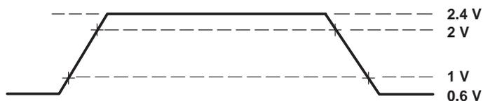
Figure 5. TTL-Level Outputs
