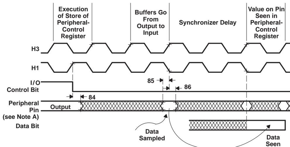
NOTE A: Peripheral pins include CLKX0, CLKR0, DX0, DR0, FSX0, FSR0, and TCLK0/1.
