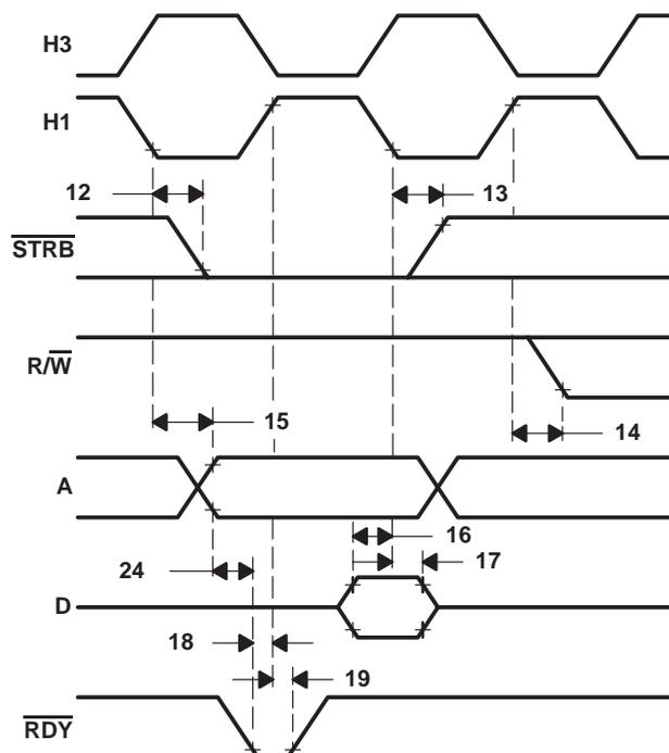
NOTE A:  $\overline{\text{STRB}}$  remains low during back-to-back read operations.
