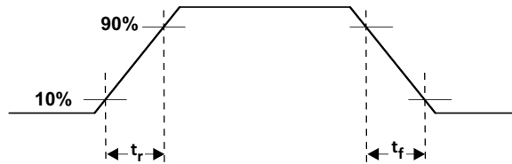
Figure 2. Output Rise and Fall Times
