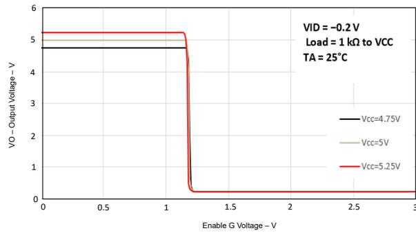
**Figure 5-7. Output Voltage vs Enable G Voltage**
