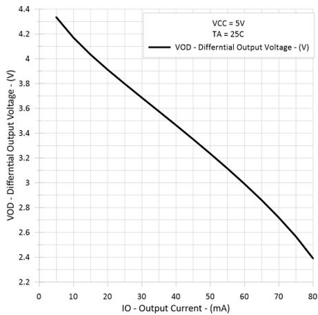
**Figure 5-3. Driver Differential Output Voltage vs Output Current**
