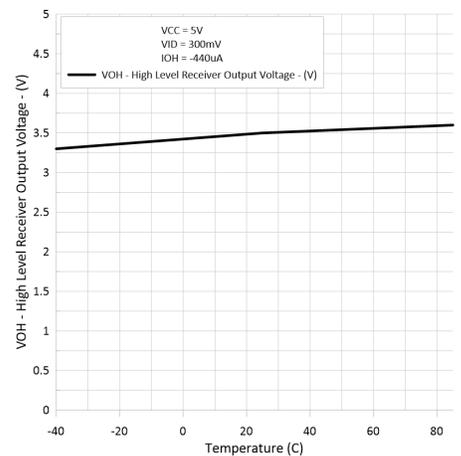
**Figure 5-5. Receiver High-Level Output Voltage vs Free-Air Temperature**
