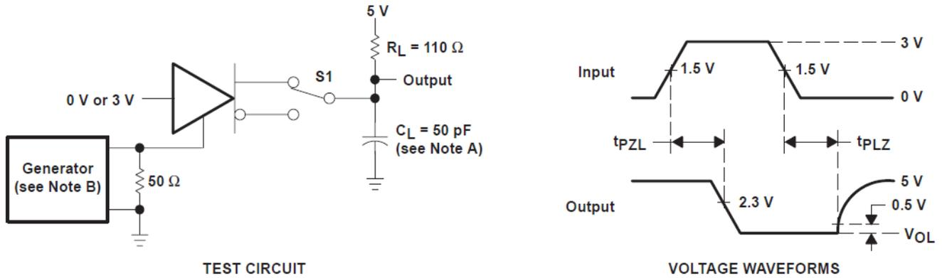
**Figure 6-5. Driver Test Circuit and Voltage Waveforms**
