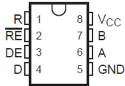
**Figure 4-1. D or P Package (Top View)**
