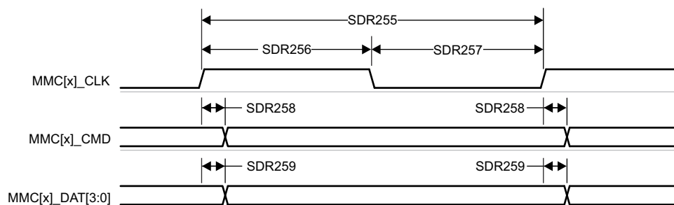
Figure 6-96. MMC1/2 – UHS-I SDR25 – Transmit Mode
