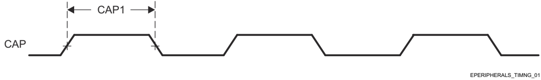
Figure 6-46. eCAP Input Timings
