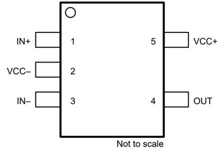
**Figure 4-2. TL071H DCK Package, 5-Pin SC70 (Top View)**
