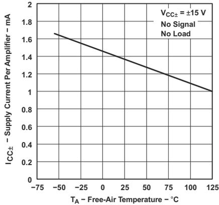
Figure 5-50. Supply Current Per Amplifier vs Free-Air Temperature
