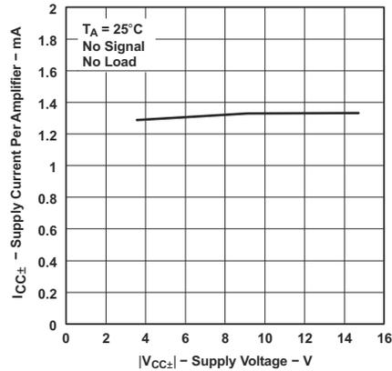
**Figure 5-49. Supply Current Per Amplifier vs Supply Voltage**
