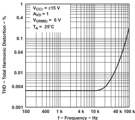
Figure 5-54. Total Harmonic Distortion vs Frequency
