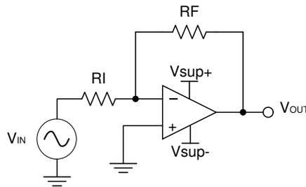
Figure 8-1. Inverting Amplifier
