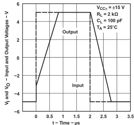
Figure 5-55. Voltage-Follower Large-Signal Pulse Response
