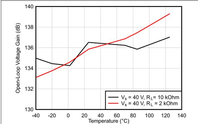
Figure 5-21. Open-Loop Voltage Gain vs Temperature
