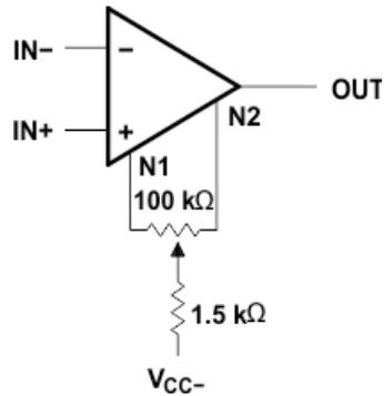
**Figure 6-3. Input Offset-Voltage Null Circuit
