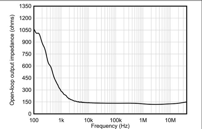
Figure 5-22. Open-Loop Output Impedance vs Frequency
