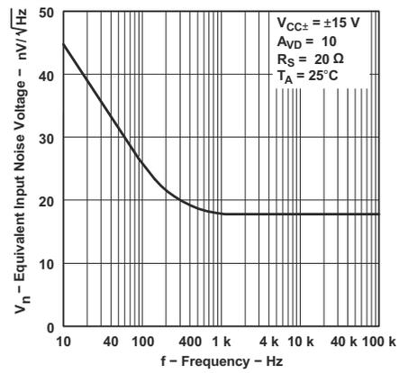
Figure 5-53. Equivalent Input Noise Voltage vs Frequency
