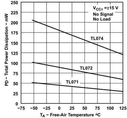
Figure 5-51. Total Power Dissipation vs Free-Air Temperature
