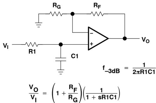
**Figure 50. Single-Pole Low-Pass Filter**
