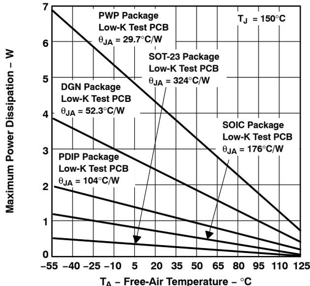
NOTE A: Results are with no air flow and using JEDEC Standard Low-K test PCB.
