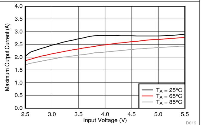
Figure 16. Maximum Output Current at V\_OUT = 1.8 V
