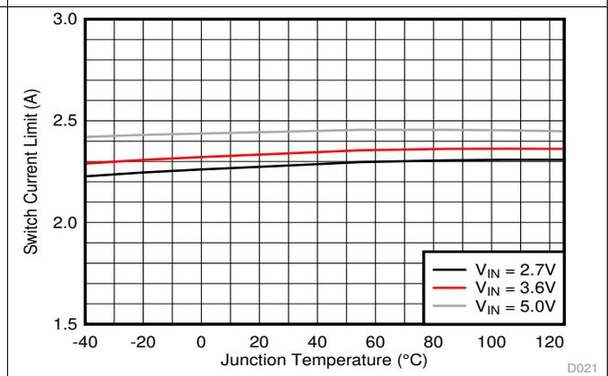
Figure 4. Switch Current Limit, TLV62568A
