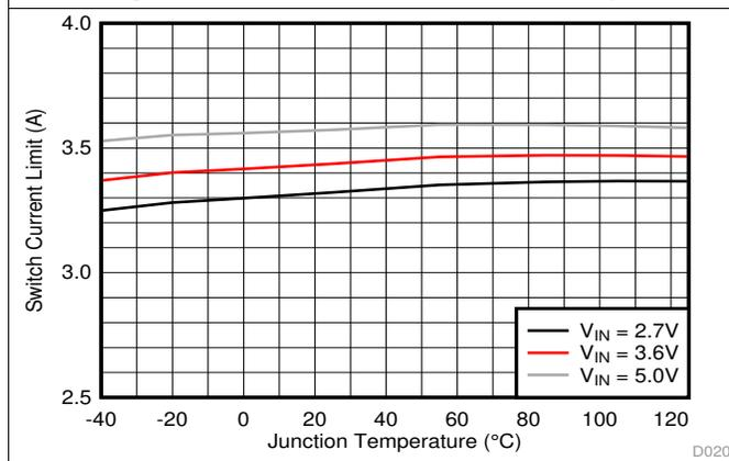
Figure 3. Switch Current Limit, TLV62569A
