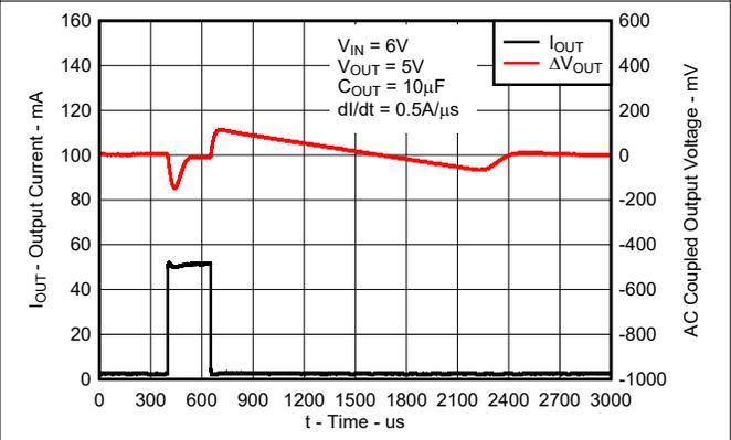
Figure 6-28. Load Transient Response for New Chip
