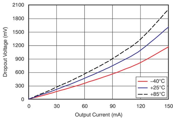
Figure 6-9. Dropout Voltage vs Output Current for Legacy Chip
