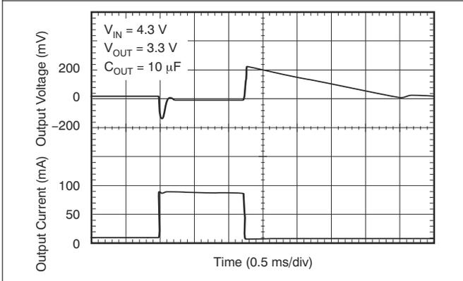
Figure 6-27. Load Transient Response for Legacy Chip
