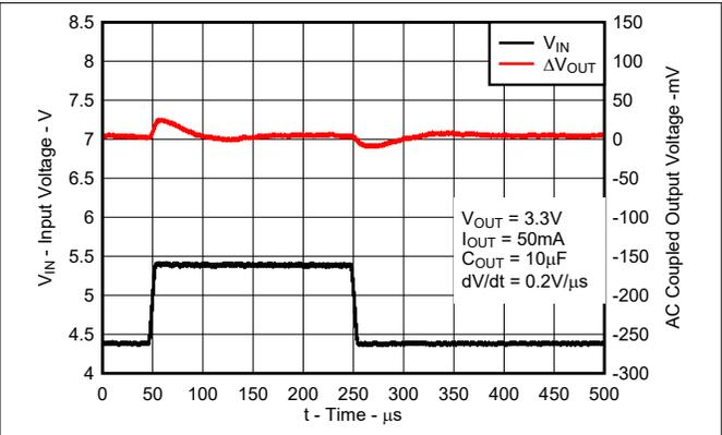
Figure 6-26. Line Transient Response for New Chip
