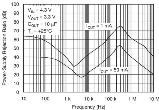
**Figure 6-21. Power-Supply Ripple Rejection vs Frequency for Legacy Chip**
