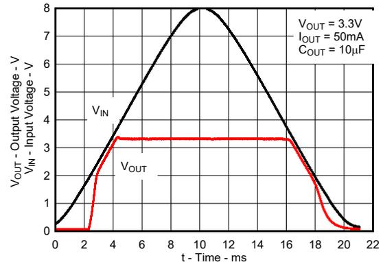
**Figure 6-24. Power-Up, Power-Down for New Chip**
