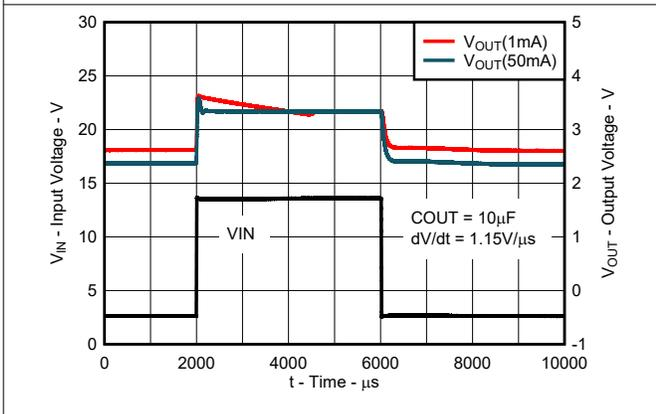
Figure 6-29. Line Transient Response for New Chip
