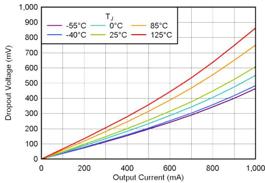
$V_{OUT} = 1.8\text{V}$ , Test condition:  $V_{IN} = V_{OUT(NOM)}$
