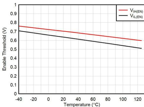
**Figure 5-11. Enable Logic Threshold vs Temperature**
