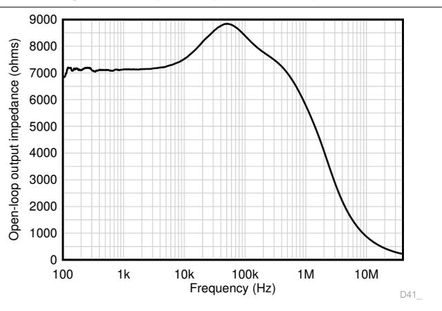
Figure 6-12. Open-Loop Output Impedance vs Frequency
