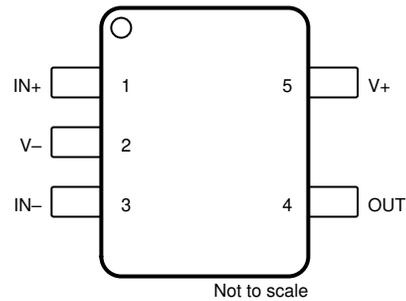
**Figure 5-2. TLV9041U DBV Package 5-Pin SOT-23 Top View**
