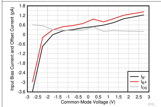
Figure 6-9.  $I_B$  and  $I_{OS}$  vs Common-Mode Voltage
