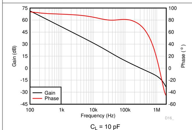
Figure 6-11. Open-Loop Gain and Phase vs Frequency
