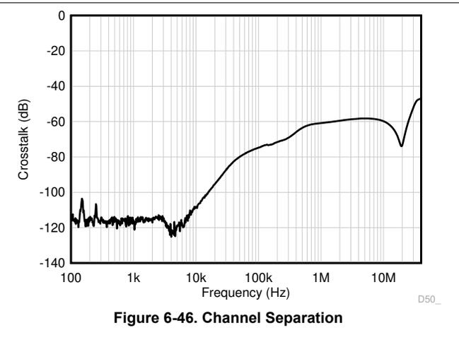
**Figure 6-46. Channel Separation**
