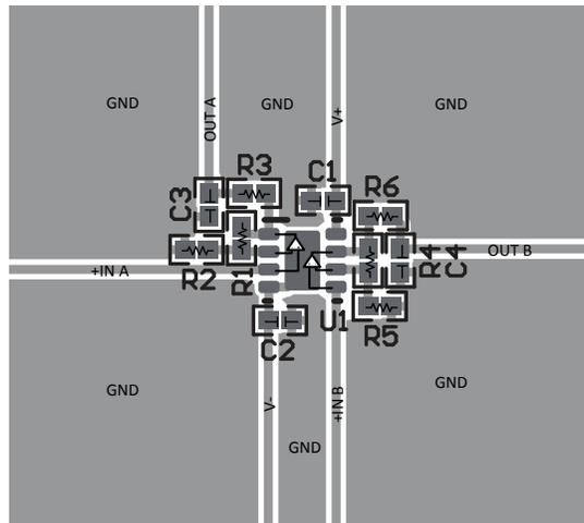
Figure 8-6. Example Layout for WSON-8 (DSG) Package
