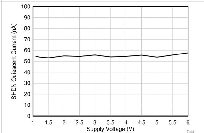
**Figure 6-41. Shutdown Mode Quiescent Current vs Supply Voltage**
