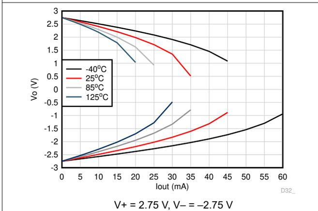
**Figure 6-15. Output Voltage vs Output Current (Claw)**
