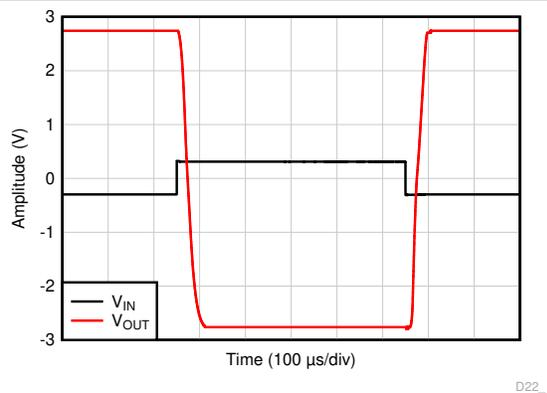
$G = -10$   $V_{IN} = 600\text{ mV}_{PP}$
