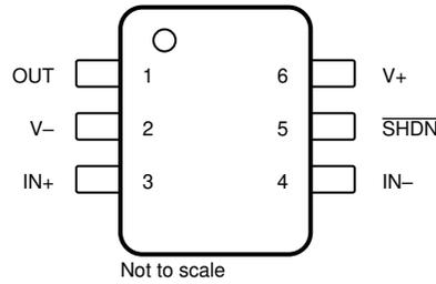
**Figure 5-5. TLV9041S DBV Package 6-Pin SOT-23 Top View**
