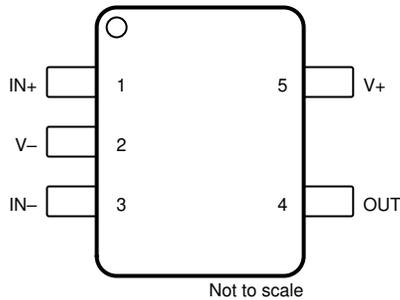
**Figure 5-3. TLV9041 DCK Package 5-Pin SC70 Top View**
