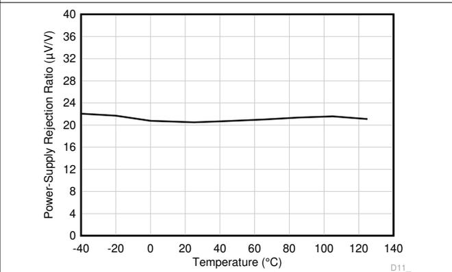
**Figure 6-18. DC PSRR vs Temperature**
