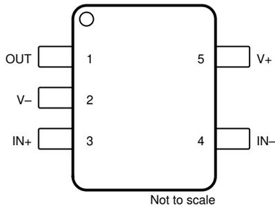
**Figure 5-1. TLV9041 DBV Package 5-Pin SOT-23 Top View**
