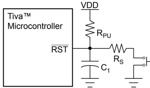
Typical  $R_{PU} = 10\text{ k}\Omega$
