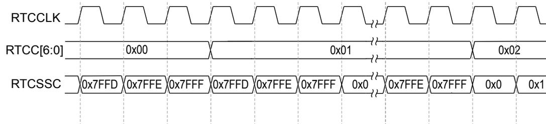
In the case of a trim value below `0x7FFF`, the `RTCSSC` value is advanced from `0x7FFF` to the trim value while the `RTCC` value is incremented from `0x0` to `0x1`. If the match value is within that range, the match interrupt is not triggered. For example, as shown in Figure 7-6 on page 485, if the match interrupt was configured with `RTCM0=0x1` and `RTCSSM=0x2`, an interrupt would never be triggered.
