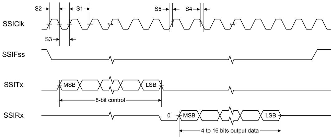
Figure 22-22. Master Mode SSI Timing for SPI Frame Format (FRF=00), with SPH=1
