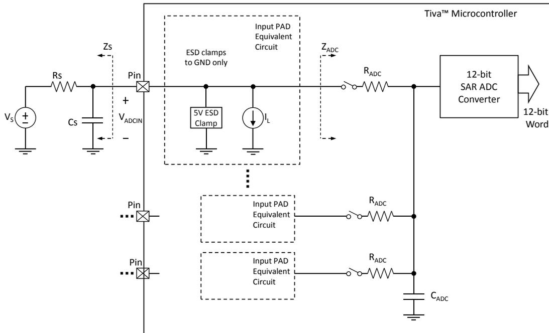
The ADC operates from both the 3.3-V analog and 1.2-V digital power supplies. The ADC clock can be configured to reduce power consumption when ADC conversions are not required (see “System Control” on page 221). The analog inputs are connected to the ADC through specially balanced input paths to minimize the distortion and cross-talk on the inputs. Detailed information on the ADC power supplies and analog inputs can be found in “Analog-to-Digital Converter (ADC)” on page 1286.
