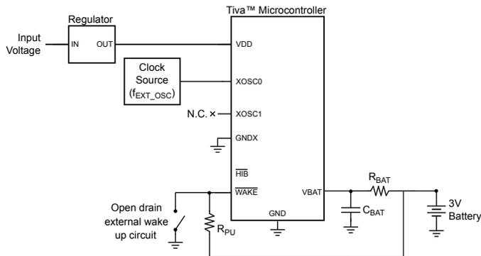
**Note:** Some devices may not supply the GNDX,  $\overline{\text{WAKE}}$  or  $\overline{\text{HIB}}$  signals. See “Signal Tables” on page 1223 for pins specific to your device.
