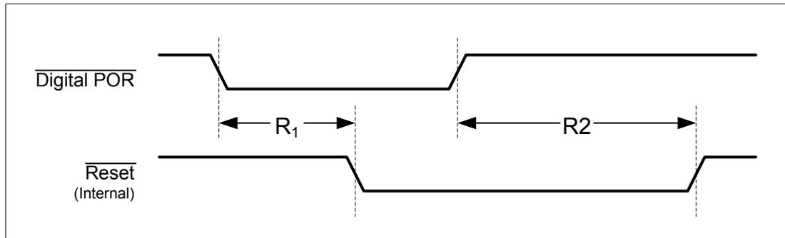
**Note:** The digital Power-On Reset is only released when the analog Power-On Reset has deasserted and all of the Power-OK monitors for each of the supplies indicate that power levels are in operational ranges.
