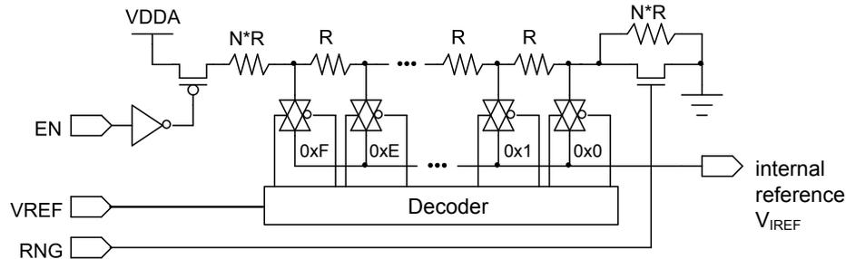
**Note:** In the figure above,  $N \cdot R$  represents a multiple of the  $R$  value that produces the results specified in Table 19-2 on page 1209.
