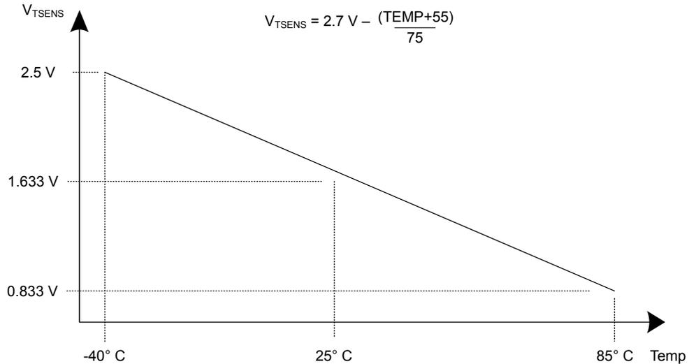
The temperature sensor reading can be sampled in a sample sequence by setting the  $TS_n$  bit in the **ADCSSCTLn** register. The temperature reading from the temperature sensor can also be given as a function of the ADC value. The following formula calculates temperature (TEMP in °C) based on the ADC reading ( $ADC_{CODE}$ , given as an unsigned decimal number from 0 to 4095) and the maximum ADC voltage range ( $V_{REFP} - V_{REFN}$ ):
