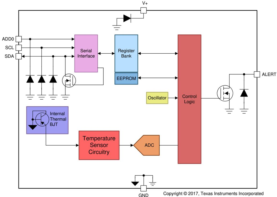
**Figure 7-1. Internal Block Diagram**
