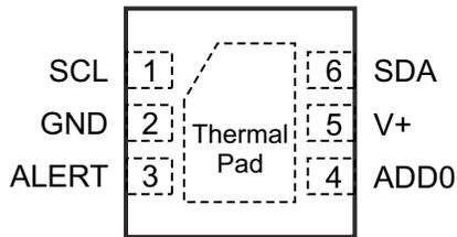
Figure 5-1. DRV Package 6-Pin WSON Top View
