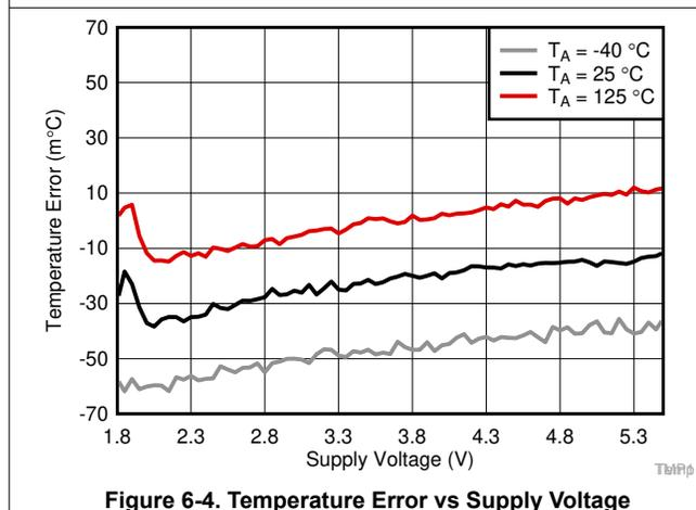
Figure 6-4. Temperature Error vs Supply Voltage
