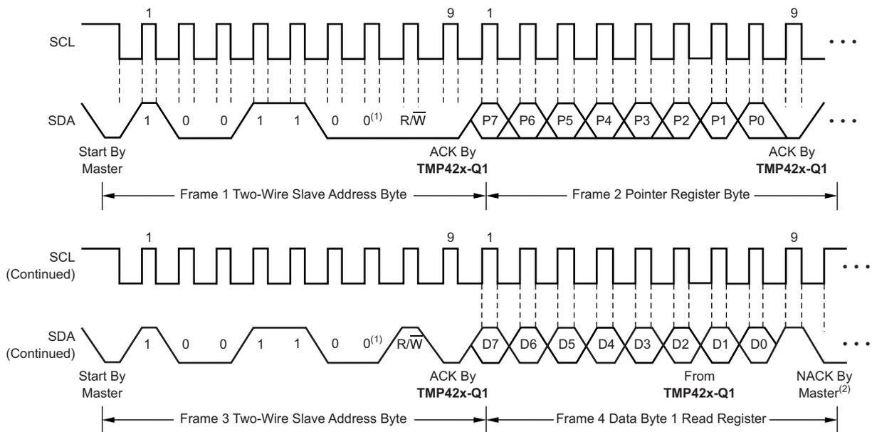
**Figure 16. Two-Wire Timing Diagram for Single-Byte Read Format**
