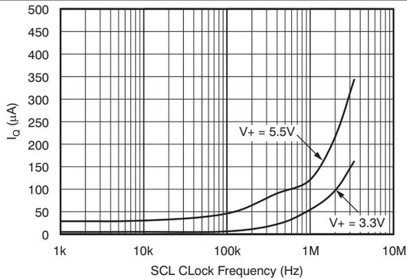
**Figure 10. Shutdown Quiescent Current vs SCL Clock Frequency**
