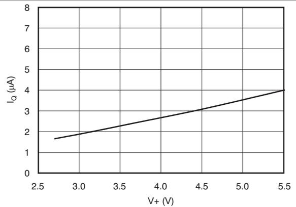
**Figure 11. Shutdown Quiescent Current vs Supply Voltage**
