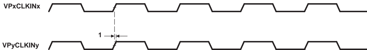
Figure 5-61. Video Port Dual-Display Sync Timing
