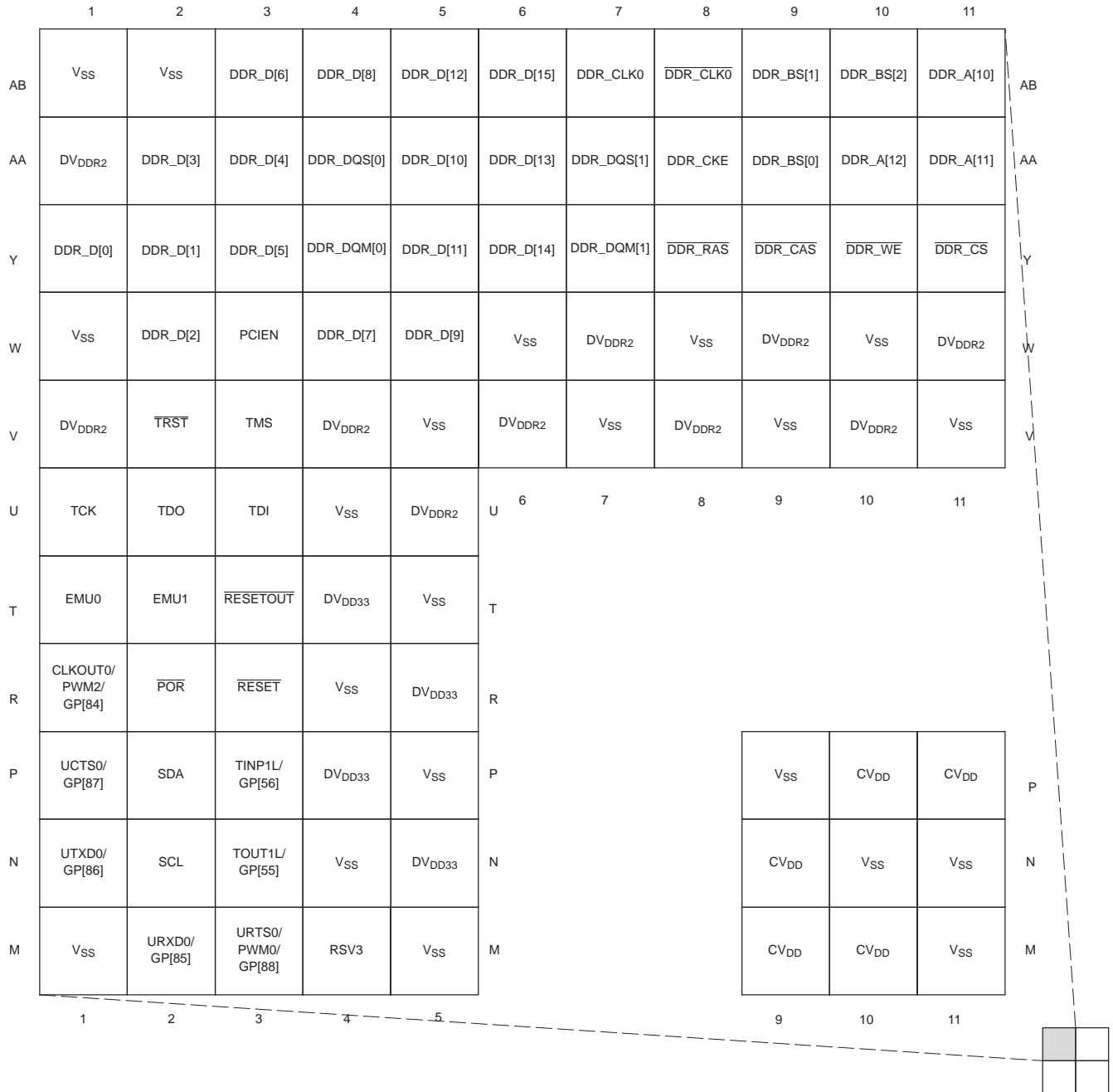
Figure 2-6. ZDU Pin Map [Quadrant A]
